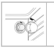
To replace the oven light bulb: 1. Remove the glass cover of the lamp-holder. 2. Remove the light bulb and replace it with a similar one: Wattage 25 W, cap E 14.
